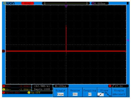
Figure 7-3 Capturing a Single Signal
