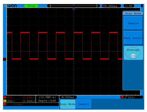
Figure 7-5 Reduce Noise level by using Average function
