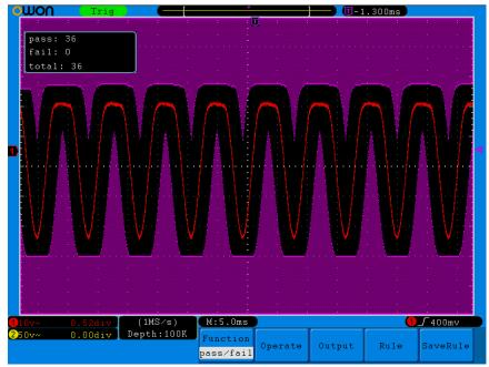
Figure 5-45 Pass/Fail test
