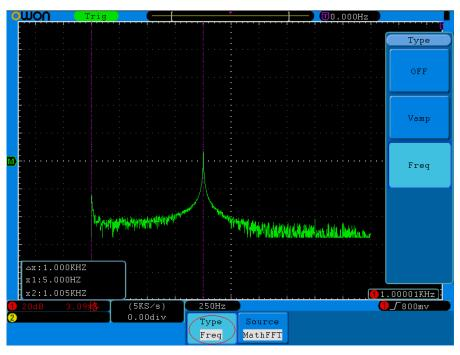
Figure 5-57 wave of Freq cursor measurement
