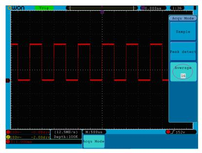
Figure 5-28 The displayed waveform after the noise is removed under the Average Mode, in which the average number of 16 is set.
