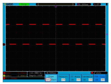
Figure 5-31 Display in Dots form
