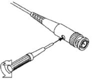
Figure 4-8 Adjust Probe
