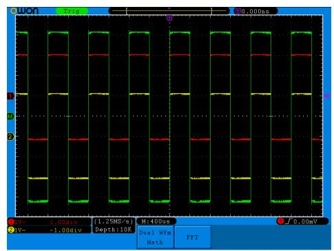
Figure 5-7 Waveform resulted from CH1 +CH2
