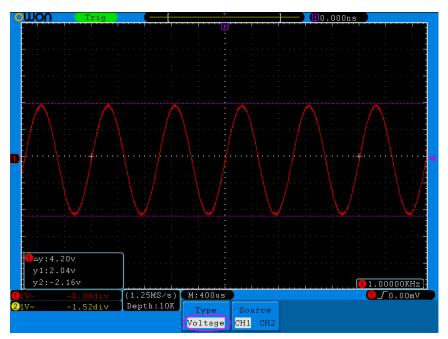
Figure 5-53 Waveform of Voltage Cursor Measurement
