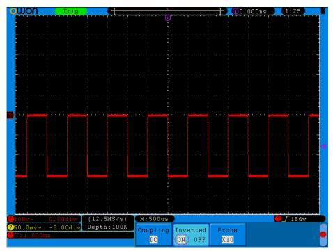
Figure 5-5 Inverted Waveform
