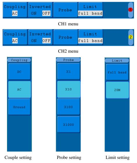
Figure 5-1 Channel Setting Menu (Only SDS7102E(V) and SDS7122E(V) have "Limit" menu)
