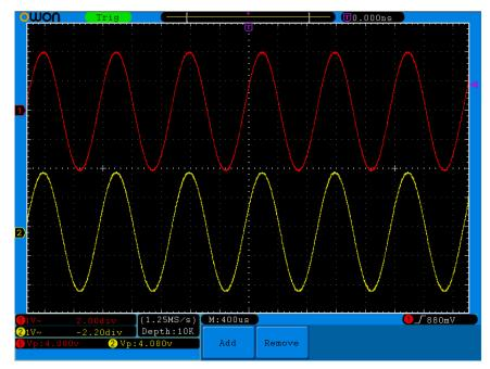
Figure 7-2 Waveform of Gain Measurement
