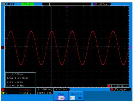
Figure 5-54 Waveform of Cursor Measurement
