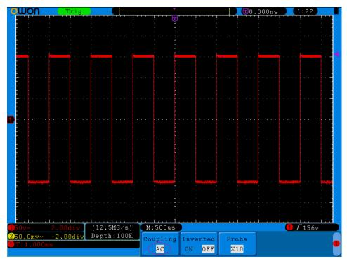
Figure 5-2 AC Coupling Oscillogram
