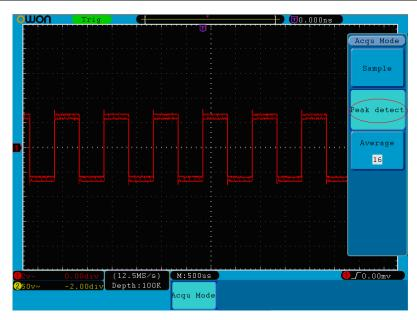
Figure 5-26 Peak Detect mode, under which the burrs on the falling edge of the square wave, can be detected and the noise is heavy.
